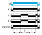
Function Dt: Symmetrical Flashing Relay (Starting Pulse Off) & With Pause / Summation Control
